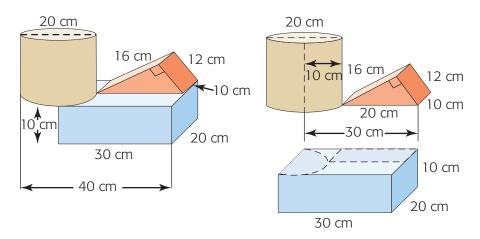
Total Surface Area = surface area of cylinder + surface area of triangular prism + surface area of rectangular prism -2 (area of semicircle) - 2(area of rectangle)
